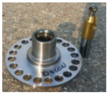
After drilling & back chamfering
